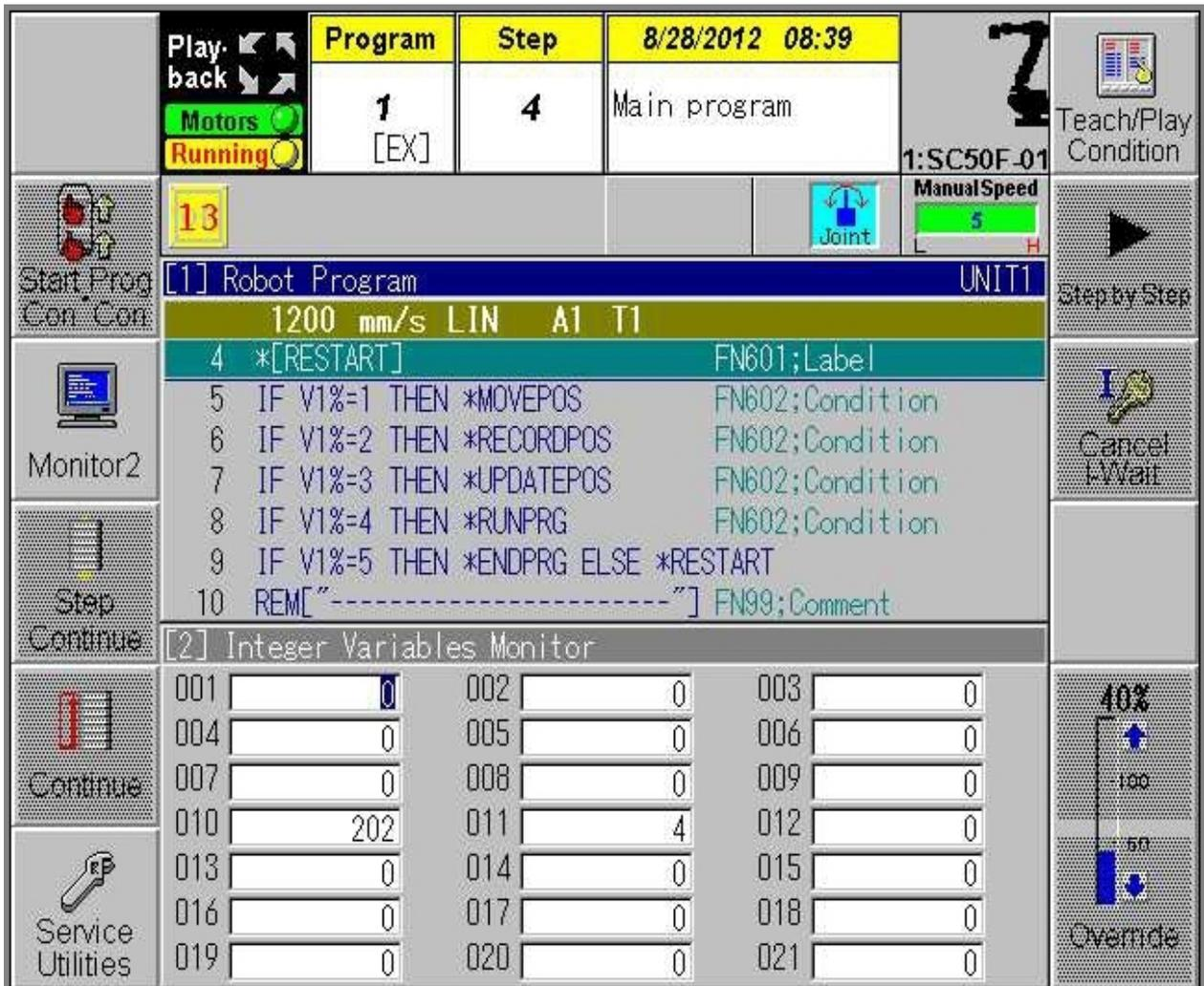
Image Display Panel during operation with a Nachi AX Controller
